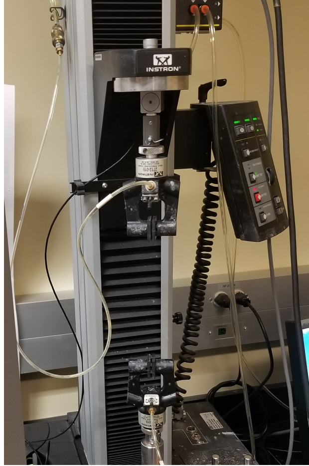
Figure 2.17: The Instron 5543A Load Frame that has been outfitted with a 100 N load cell.
