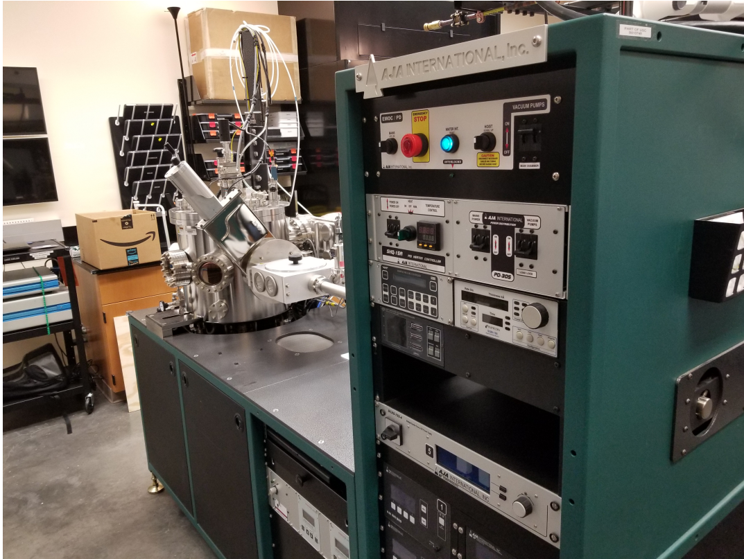
Figure 2.3: An AJA Orion sputtering chamber. This system has five sputter guns, and three target materials can be co-deposited during a single experiment.
