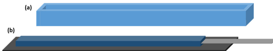
Figure 2.16: A depiction of the mold and samples for the peel test measurements. (a) The Teflon mold. (b) Example of the sample on the substrate with an aluminum mesh for gripping.
