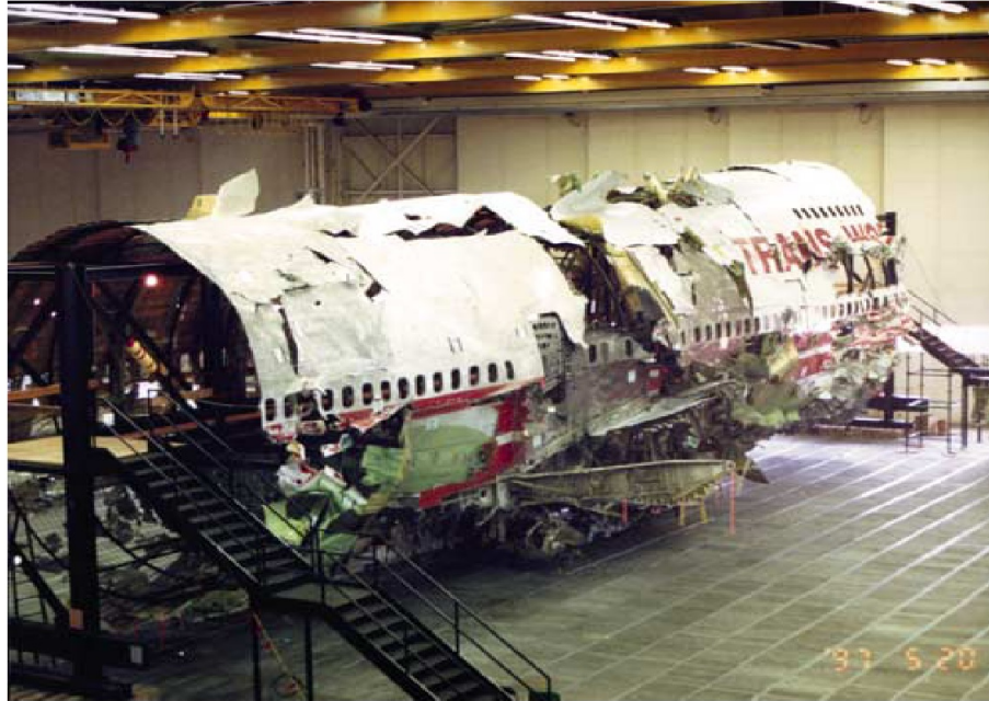
Figure 7.1: The reconstructed wreckage of flight TWA 800. [175]. 1
